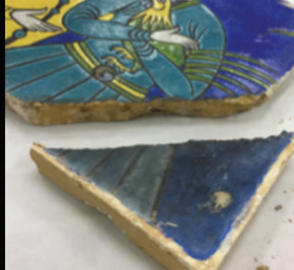
The old filler was easily detached from the tile body
